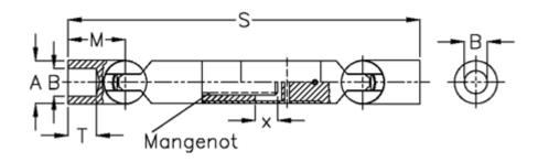
Α = 70 B H7 = 45 Longitudinal ribs = 18x44x52Μ = 105.0= 820 MD max N m = 580 = 52 Τ = 90
